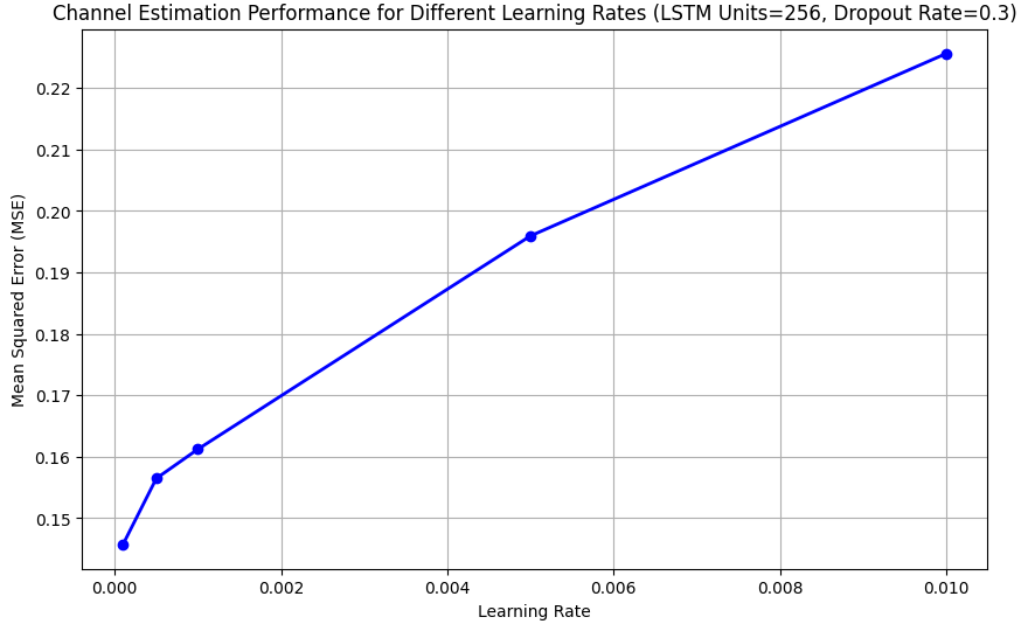
Figure 5.17: Impact of Varying Learning Rate on Channel Estimation Performance with Fixed LSTM Units (256) and Dropout Rate (0.3)
