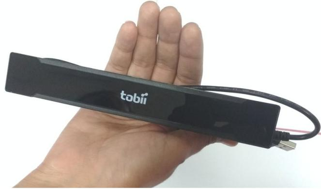
Figure 2.3: A prototype PCCR eye-tracker, Tobii X2-60
