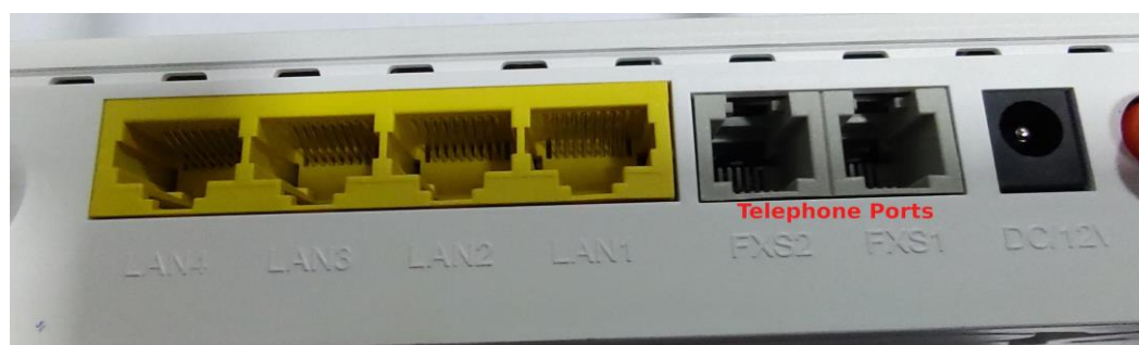
Fig: LAN and Telephone ports
