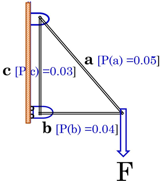
Find the probability of failure of the truss ?
