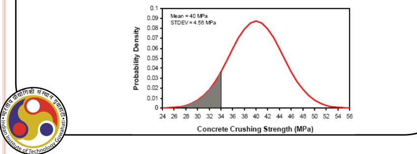
• The probability that the concrete strength is less than or equal to the applied stress (34 MPa) is obtained using the Standard Normal CDF as
