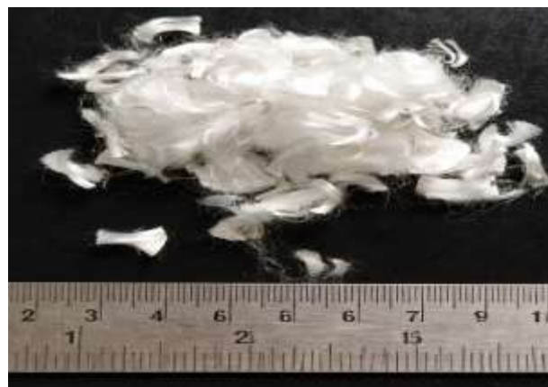
Fig. 3 PP fibers used in the study (length=12 mm), illustrating the geometry and form of discrete reinforcement employed for improving soil strength and FT resistance
