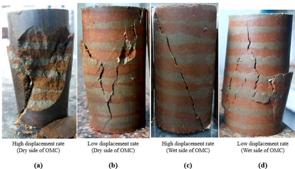
Figure 13. Failed 16L reconstituted varved clay samples after UCS test under varying displacement rates and moisture content
