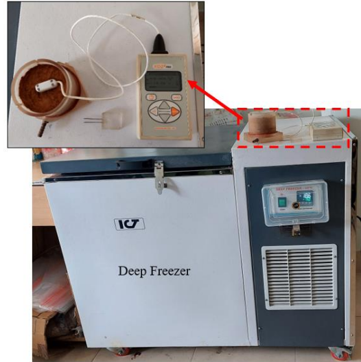
Figure 5. Measurement of thermal properties using KD2 Pro on prepared samples immediately after removal from the deep freezer
