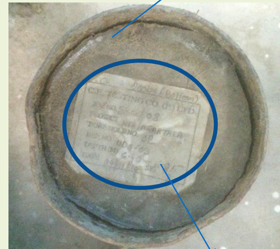
Undisturbed sample cores obtained from the site location
