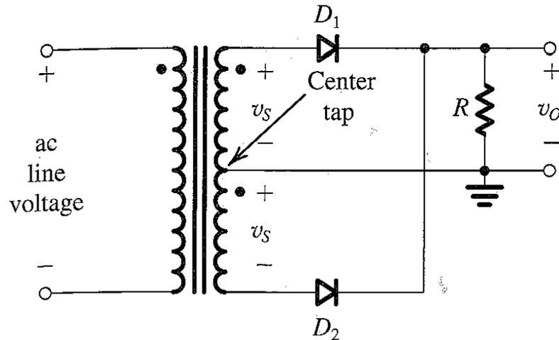
To find the PIV of the diodes in the full-wave rectifier circuit, consider the situation during the positive half-cycles. Diode  $D_1$  is conducting, and  $D_2$  is cut off. The voltage at the cathode of  $D_2$  is  $v_o$ , and that at its anode is  $-v_s$ . Thus the reverse voltage across  $D_2$  will be  $(v_o + v_s)$ , which will reach its maximum when  $v_o$  is at its peak value of  $(V_s - V_D)$ , and  $v_s$  is at its peak value of  $V_s$ ; thus,
