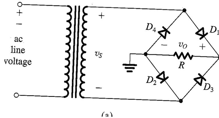
To determine the peak inverse voltage (PIV) of each diode, consider the circuit during positive half-cycles. The reverse voltage across  $D_3$  can be determined from the loop formed by  $D_3$ ,  $R$ , and  $D_2$  as
