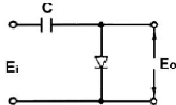
➤ During the –ve cycle when diode is reverse bias, the diode becomes to its off state. In this case, the output voltage equals to the sum of the input voltage and the voltage across the terminals of the capacitor which have the same polarity with each other
