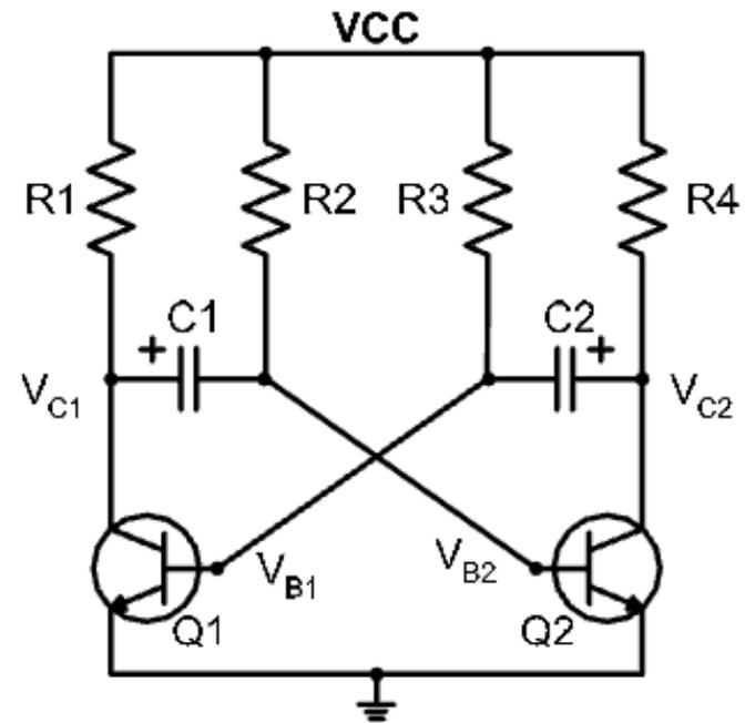
Consists of two amplifying devices cross-coupled by resistors and capacitors. Typically,  $R2 = R3$ ,  $R1 = R4$ ,  $C1 = C2$  and  $R2 \gg R1$ .
