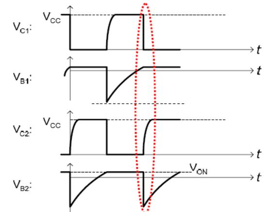
➤ Since Q1 conducts and Q2 off hence  $V_{C1} = 0V$  and  $V_{C2} = V_{CC}$ . Due to higher voltage at  $V_{C2}$ , capacitor  $C_2$  will be charged via  $R_4$  (low resistance path because  $R_4 < R_2$ ).  $C_1$  (which was charged earlier, and can not hold the charge for indefinite period) starts discharging via  $R_2$  (high resistance path because  $R_2 > R_1$ ). Time taken to discharge  $C_1$  ( $T_1 = R_2 C_1$ )  $>$  time taken to charge  $C_2$  ( $T_2 = R_4 C_2$ )
