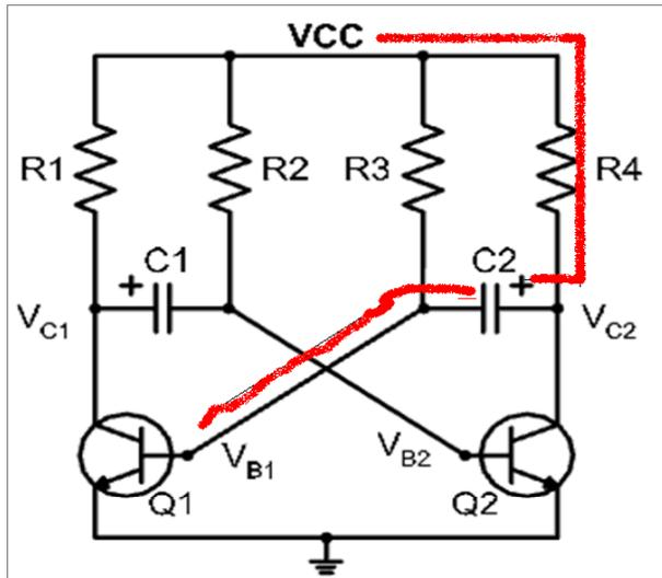
Discharging  $C_1$  ( $T_1 = R_2 C_1$ )
