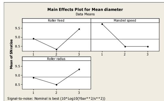
**Figure 3 Main effects plot for mean diameter**
