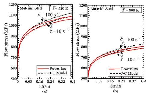
**Figure 6** Variation of flow stresses with strain for steel at actual and estimated material properties at temperatures (a) 520 K and (b) 800K
