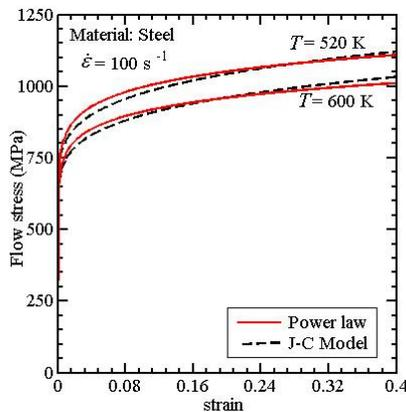
**Figure 7 Variation of flow stresses with strain at actual and estimated material properties of steel at temperatures (a) 520 K and (b) 600 K**
