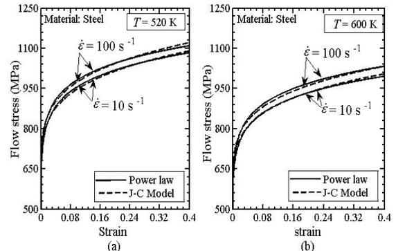
**Figure 4** Variation of flow stresses with strain for steel at actual and estimated material properties at temperatures (a) 520 K and (b) 600K
