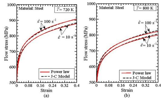
**Figure 5** Variation of flow stresses with strain for steel at actual and estimated material properties at temperatures (a) 720 K and (b) 800K
