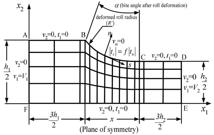
Figure 2 A meshed domain of strip with boundary conditions
