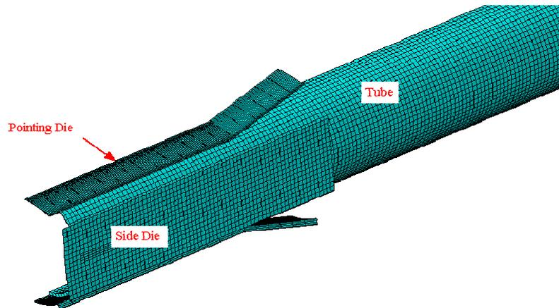
Fig.2 3D Finite Element model- Pointing
