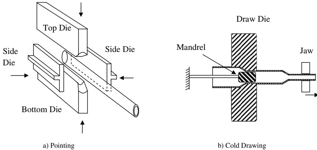
Fig.1. Cold drawing process
