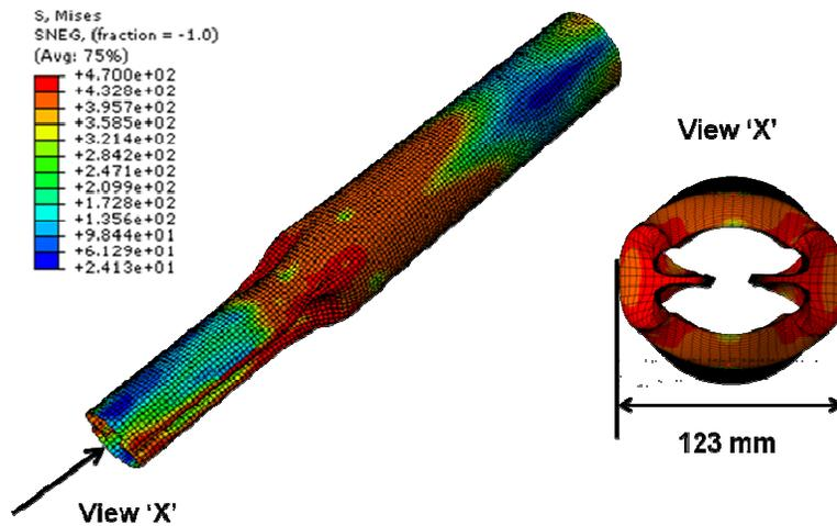
**Fig. 4 Deformed shape of after pointing operation of tube (114.3 Outer diameter)**
