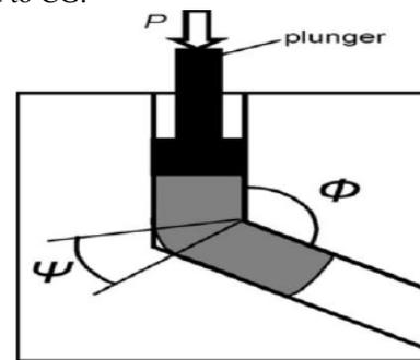
**Fig. 3 Die drawing for Schematic representation of ECAP process** (V M Segal 1995).
