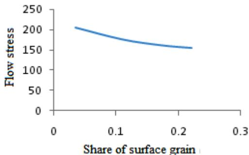
Fig. 8 Flow stress with share of surface grain (U Engel et al. 2001).
