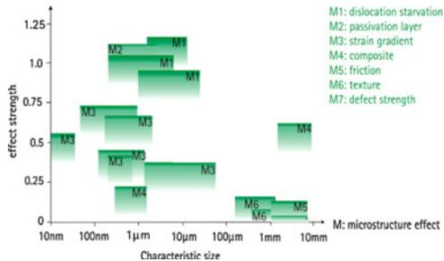
**Fig. 11 Strength of material with microstructure size** (F. Vollertsen et al. 2009).
