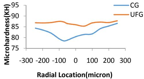
**Fig. 13 micro hardness of CG and UFG (a) before and (b) after extrusion** (Sunal Ahmet Parasız et al. 2011).
