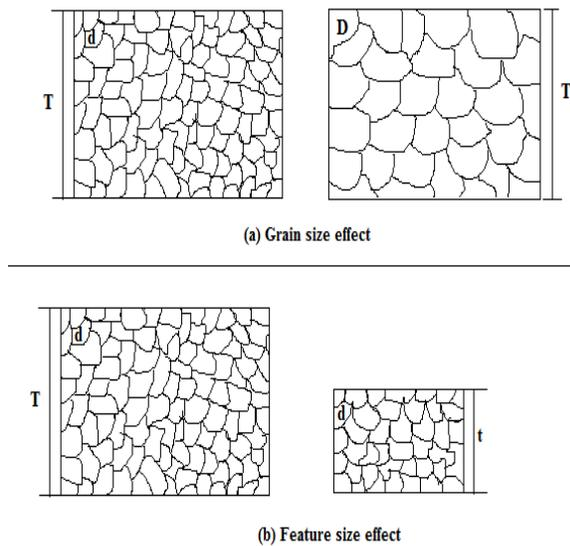
**Fig. 5 (a) Grain size effects and (b) feature size effects with the decreasing of scale (Xinmin Lai et al. 2008).**
