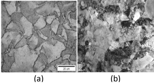
Fig. 7 structure of (a)CG and (b)UFG (S. Geißdörfer et al. 2008).
