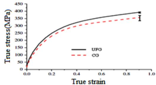
Fig. 9 Flow stress-strain curve (W.L. Chan et al. 2011).
