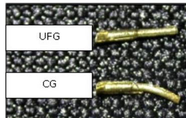
Fig. 10 Flow pattern of CG and UFG sample (Sunal Ahmet Parasız et al. 2011).
