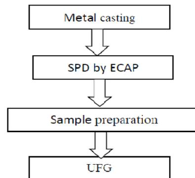
**Fig. 4 Flow chart for UFG microstructure preparation**
