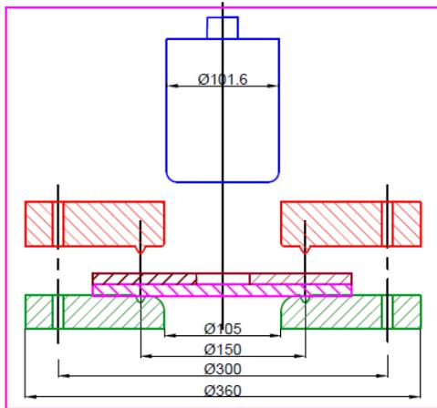
Figure 2 Set-up for biaxial pre-strain (Step- I)
