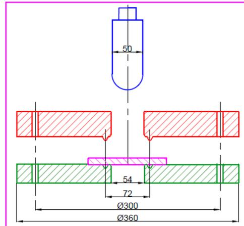
Figure 3 Out-of-plane stretch forming (Step- II)
