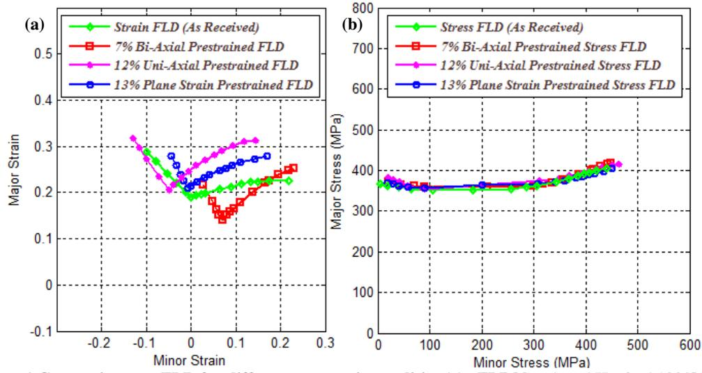
Figure 1 Conversion to  $\sigma$ -FLD for different pre-strain condition (a)  $\epsilon$ -FLD [Graph and Hosford, 1993] (b)  $\sigma$ -FLD
