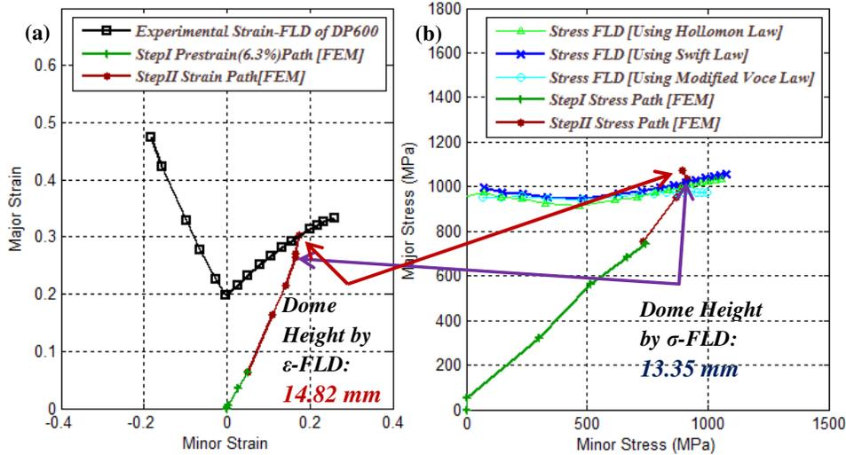
Figure 5 (a) Strain and (b) stress path during forming of 6.3% pre-strained DP600 material
