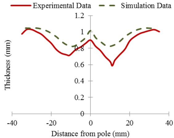
Figure 7 Thickness distribution in a stretch formed cup from 6.3% pre-strained DP600 metal
