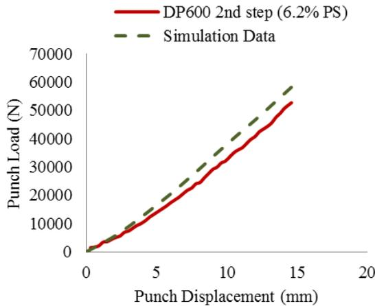
Figure 6 Load-displacement curve during deformation of 6.3% pre-strained DP600 metal
