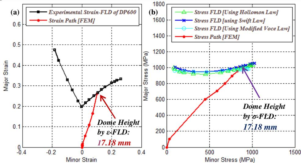
**Figure 4 (a) Strain and (b) stress path during forming of DP600 as received material**
