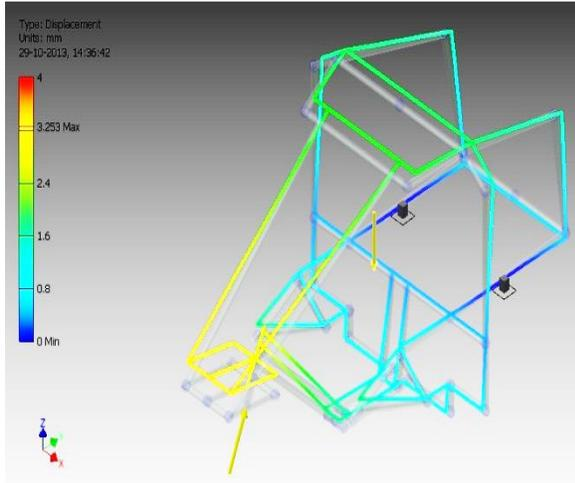
**Figure 5 Front bump test**
