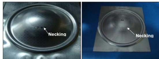
Figure 5: Necking in the samples
