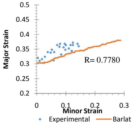
**Figure 7: Comparison of FLD based on Barlat with experimental FLD results and the corresponding R value**
