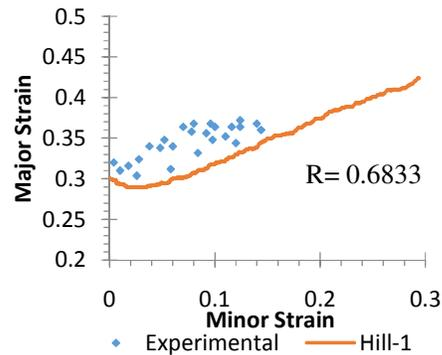
Figure 5: Comparison of FLD based on Hill-1 with experimental FLD results and the corresponding R value
