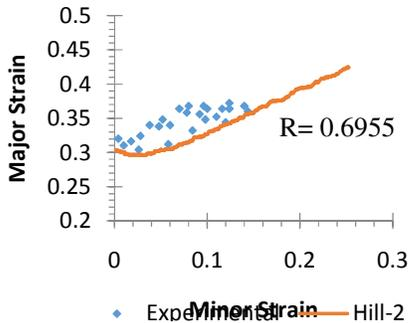
**Figure 6: Comparison of FLD based on Hill-2 with experimental FLD results and the corresponding R value**
