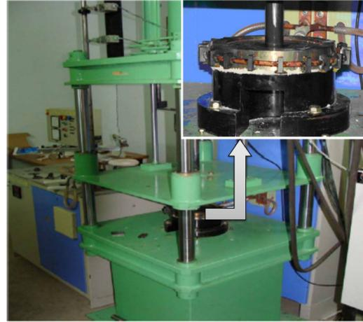
**Figure 1: Hemispherical dome test setup**
