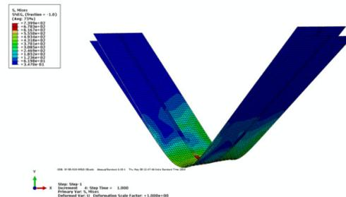
**Figure 7 F.E. simulation of V-bending showing springback in TWBs**
