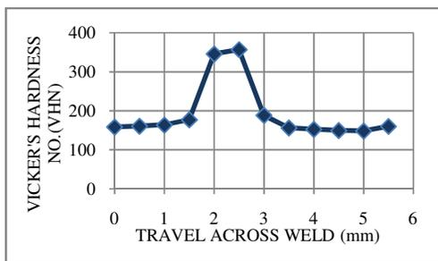
**Figure 1 Variation of micro hardness across the weld region**
