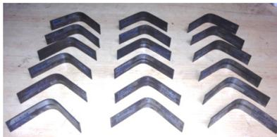
**Figure 6 Tested bend specimens of TWBs with three thickness combinations**
