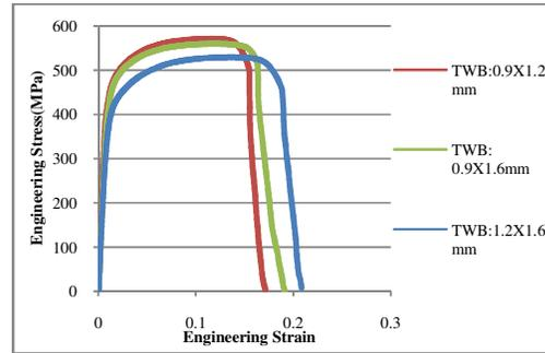
Figure 9 Engineering stress - strain curves of the weld zone with three thickness combinations
