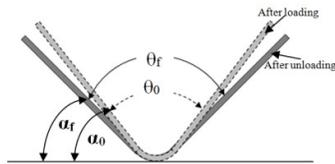
**Figure 5 Measurement of springback**
