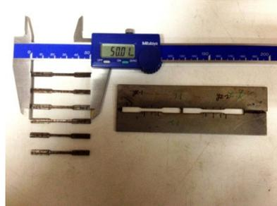
**Figure 2 Tensile specimens of weld zone**
