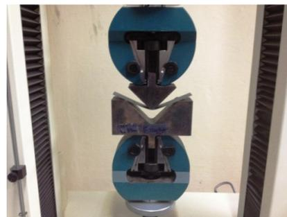
**Figure 4 Experimental set-up for determination of springback in V-bending**
