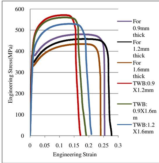
Figure 8 Engineering stress - strain curves of high strength steel and TWBs samples
