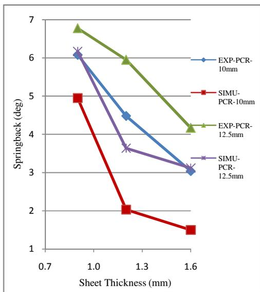
Figure 10 Experimental and simulation results for springback for parent materials
