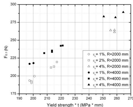
Figure 5: The dent resistance force as a function of the panel yield strength multiplied by the panel thickness.
