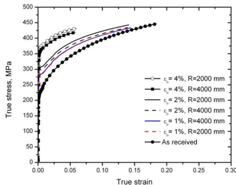
**Figure 8: Effect of back hardening on Mechanical properties**
