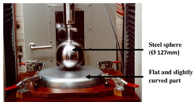
**Figure 1: Static Dent Resistance Test Setup**
