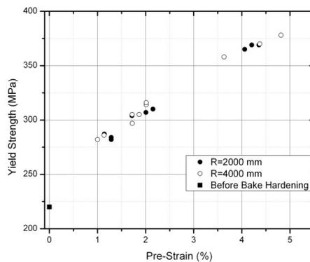
**Figure 6: Effect of pre-strain on yield strength after bake hardening**
