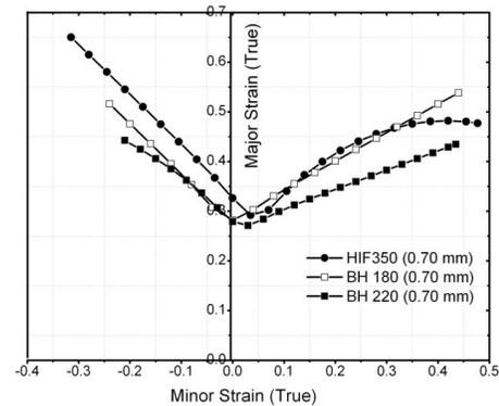
Figure 4: Forming Limit Diagram
