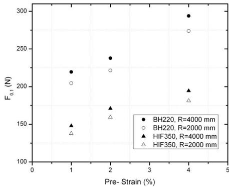
**Figure 11: Calculated dent resistance force with SDR regression formulae**
