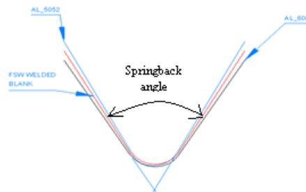
**Figure 4** Representation of relative spring back of base materials and welded sheets
