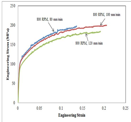
**Figure 2** Tensile behaviour of weld zone at different welding speeds
