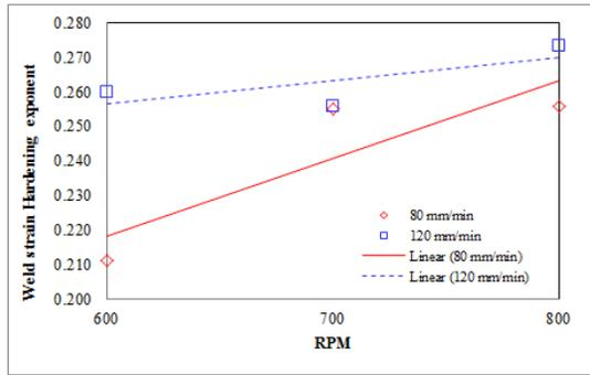
**Figure 6** Effect of rotational speed and welding speed on weld zone ‘n’ value (Error in *n*: 0.002)
