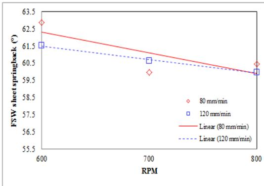
**Figure 7** Effect of rotational speed and welding speed on springback of FSW sheets (Error in angle: 1.2°)
