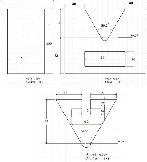
Figure 1 Schematic of die and punch in V-bending setup
