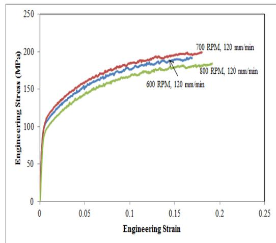
**Figure 3** Tensile behaviour of weld zone at different rotational speeds
