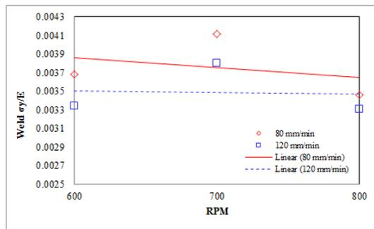
**Figure 5** Effect of rotational speed and welding speed on  $\sigma_y/E$  ratio of weld zone (Error in  $\sigma_y/E$ : 0.0001)
