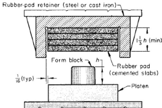
Fig1: Set up for rubber forming by Guerin Process
