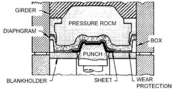
Fig 3: Verson-Hydroform process
