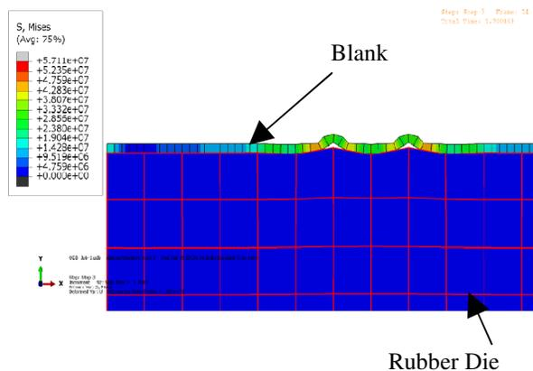
Figure 5: Von Mises stress plot after forming
