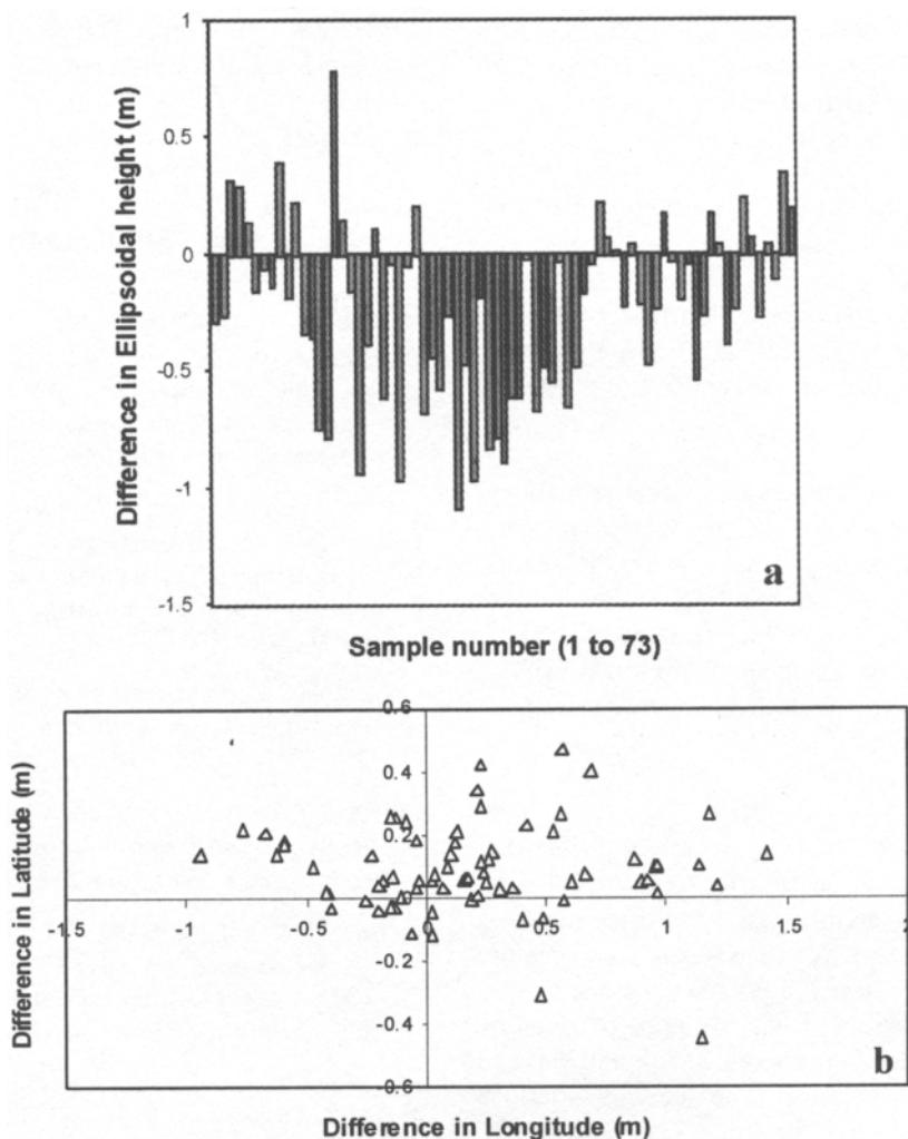
**Fig. 4.** Error in coordinates of IITK reference station estimated from 30 minute GPS observation for 73 samples: 4(a) Ellipsoidal height; 4(b) Latitude and Longitude.
