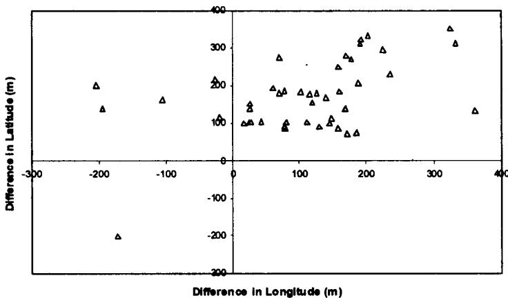
Fig. 3. Difference of estimated-in-laboratory and measured-in-field coordinates for 46 points.
