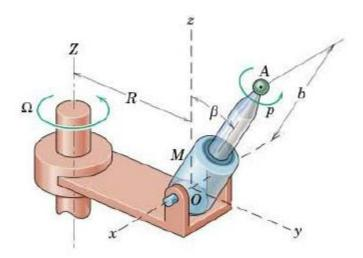
**Ques.2** – The circular disk of 100-mm radius rotates about its *z*-axis at the constant speed p = 240 rev/min, and arm OCB rotates about *Y*-axis at the constant speed N = 30rev/min. Determine the velocity **v** and acceleration **a** of point *A* on the disk as it passes the position shown. Use reference axes *x*-*y*-*z* attached to arm OCB.
