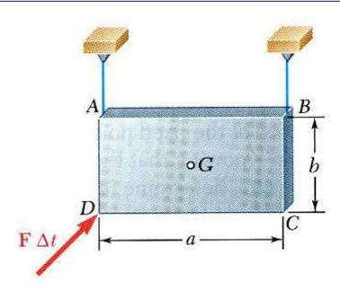
Rectangular plate of mass *m* that is suspended from two wires is hit at *D* in a direction perpendicular to the plate.
