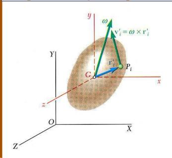
$$\begin{split} H_{x} &= + \bar{I}_{x} \omega_{x} - \bar{I}_{xy} \omega_{y} - \bar{I}_{xz} \omega_{z} \\ H_{y} &= - \bar{I}_{yx} \omega_{x} + \bar{I}_{y} \omega_{y} - \bar{I}_{yz} \omega_{z} \\ H_{z} &= - \bar{I}_{zx} \omega_{x} - \bar{I}_{zy} \omega_{y} + \bar{I}_{z} \omega_{z} \end{split}$$
