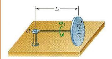
A homogeneous disk of mass m is mounted on an axle OG of negligible mass. The disk rotates counter-clockwise at the rate  $\omega_1$  about OG.
