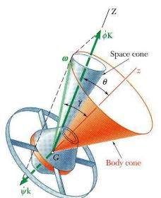
The motion of a body about a fixed point (or its mass center) can be represented by the motion of a body cone rolling on a space cone. In the case of steady precession the two cones are circular.
