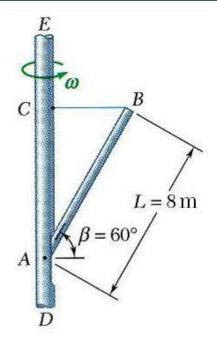
Rod AB with weight W = 40 N is pinned at A to a vertical axle which rotates with constant angular velocity  $\omega = 15 \text{ rad/s}$ . The rod position is maintained by a horizontal wire BC.
