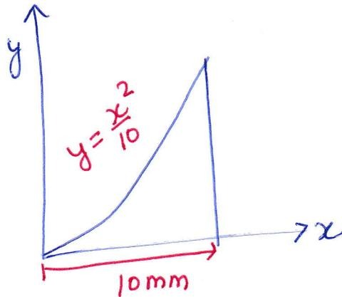
Step 1 For calculation of  $I_{xx}$ , use a horizontal strip of width  $dy$  as shown
