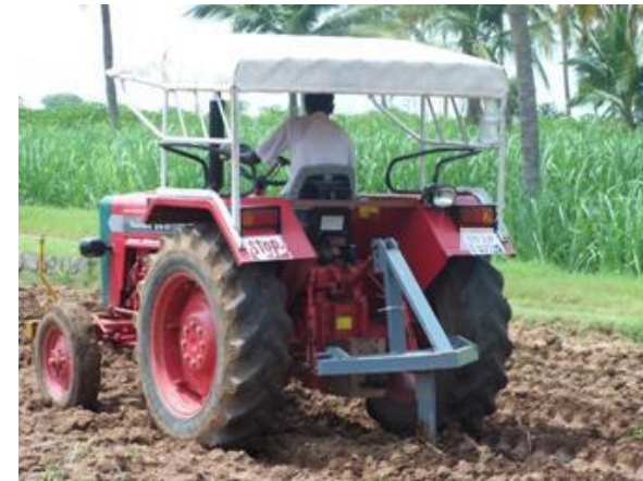
Large Rolling Resistance due to wet field
