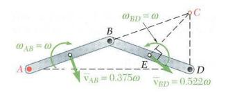
• Express the final kinetic energy of the system in terms of the angular velocities of the rods.
