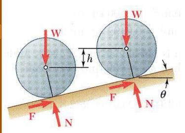
• Because each of the bodies has a different centroidal moment of inertia, the distribution of the total kinetic energy between the linear and rotational components will be different as well.
