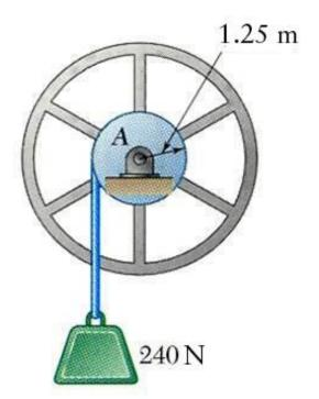
For the drum and flywheel,  $\bar{I} = 10.5 \text{ kgm}^2$ The bearing friction is equivalent to a couple of  $60 \text{ N} \cdot \text{m}$  At the instant shown, the block is moving downward at 6 m/s
