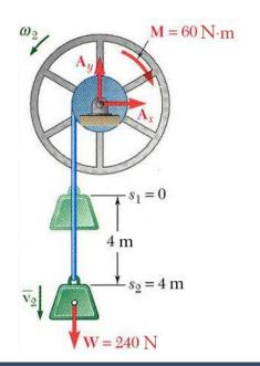
$$T_1 = \frac{1}{2}mv_1^2 + \frac{1}{2}\bar{I}\omega_1^2 = 552.96 \text{ N} \cdot \text{m}$$
