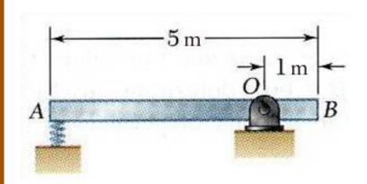
A 30-N slender rod pivots about the point O. The other end is pressed against a spring (k = 1800 N/m) until the spring is compressed 30 cm and the rod is in a horizontal position.
