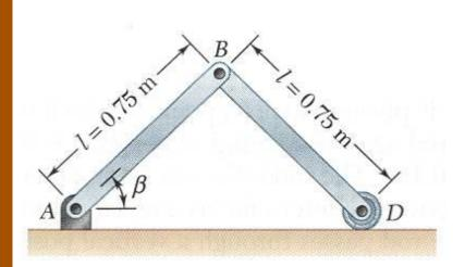
Each of the two slender rods has a mass of 6 kg. The system is released from rest with  $\beta = 60^{\circ}$ .
