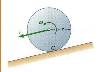
A sphere, cylinder, and hoop, each having the same mass and radius, are released from rest on an incline. Determine the velocity of each body after it has rolled through a distance corresponding to a change of elevation h.
