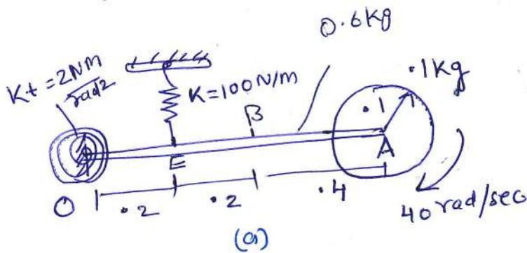
The hinge at A is frictionless and there is constant frictional torque of 0.1 Nm on the rod from hinge at O.
