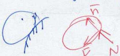
4. Reaction  $\vec{R}$  at A at smooth ball and socket or smooth hinge joint with a fixed body since  $\dot{W} = \vec{R} \cdot \vec{v}_A = \vec{R} \cdot \vec{0} = 0$
