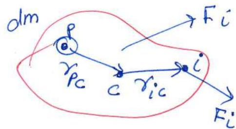
$$= \frac{1}{2} m \bar{v}_c \cdot \bar{v}_c + \frac{1}{2} \int_m \bar{v}_{pc} \cdot \bar{v}_{pc} dm$$
