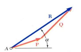
Graphical solution - A triangle is drawn with P and Q head-to-tail and to scale. The magnitude and direction of the resultant or of the third side of the triangle are measured,
