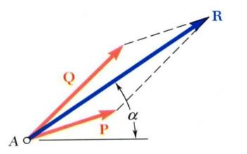
Graphical solution - A parallelogram with sides equal to P and Q is drawn to scale. The magnitude and direction of the resultant or of the diagonal to the parallelogram are measured,
