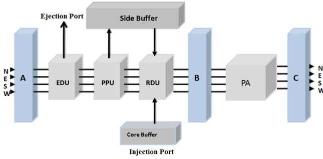
**Figure. 4:** Deflection Router Architecture that supports multicasting.
