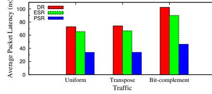
Figure 12. Comparative analysis of average packet latency for various traffics in 4x4 mesh NoC at pre-saturated load (DR:Distributed XY Routing, ESR: Existing Source Routing, PSR: Proposed Source Routing).
