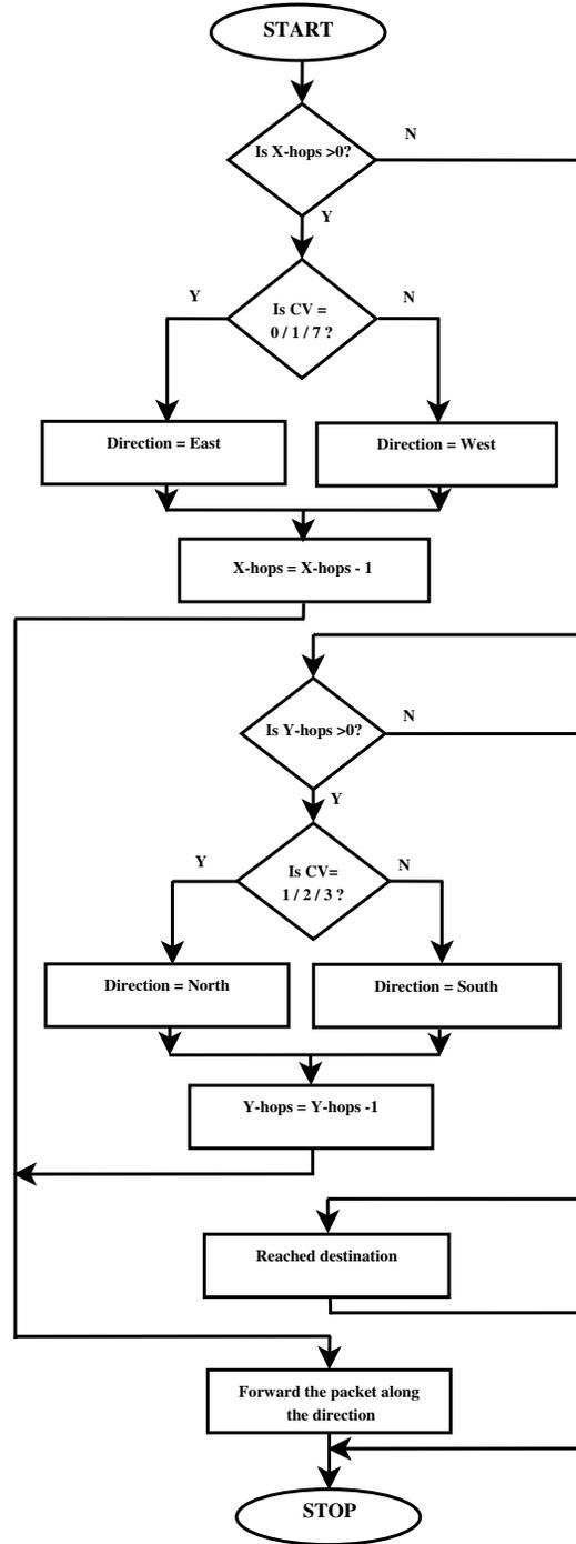
Figure 9. Route Extraction (RE) Process (Input is Route String and Output is next hop direction).
