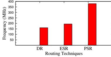
Figure 10. Comparative analysis of maximum network frequency using various routing techniques (DR: Distributed XY Routing, ESR: Existing Source Routing, PSR: Proposed Source Routing).
