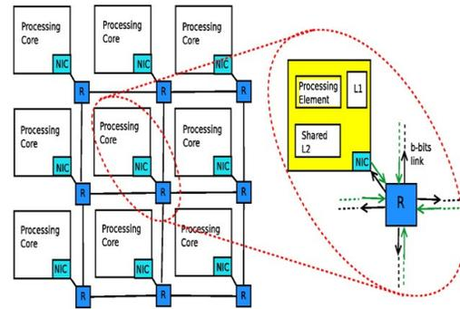
Figure 1. Processing core- router interaction in a 2D-mesh topology.
