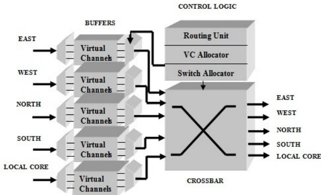
Figure 2. Conventional input buffered router.
