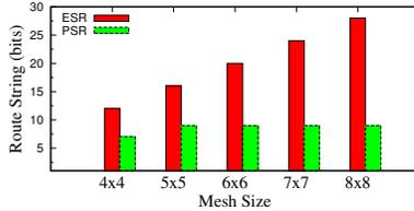
Figure 11. Comparative analysis of route string size needed for various source routing techniques (ESR: Existing Source Routing, PSR: Proposed Source Routing).
