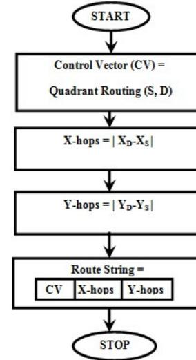
Figure 8. *Route Computation* (RC) Process (Input is Source Node-  $S(X_S, Y_S)$  and Destination Node-  $D(X_D, Y_D)$ ; Output is *Route String*).
