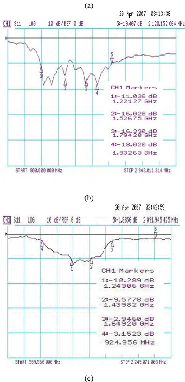
Fig. 3. (a) Photograph of the fabricated printed rectangular monopole antenna (backside view) (b) Experimental results of fabricated printed rectangular monopole for dual-band applications ( $S_{11}$  vs frequency). (c) Experimental results of fabricated printed rectangular monopole for penta-band applications ( $S_{11}$  vs frequency)
