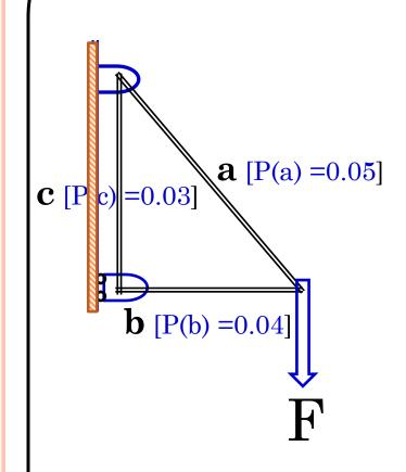
Find the probability of failure of the truss ?
