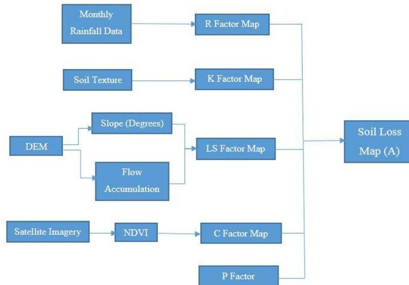
Figure 4.1 : Flowchart of RUSLE soil loss estimation using GIS and remote sensing technique
