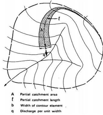
Figure 4.2 : Schematic representation of specific catchment area
