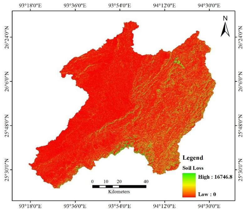
Figure 6.1 : Spatially distributed soil loss Map of Dhansiri Watershed
