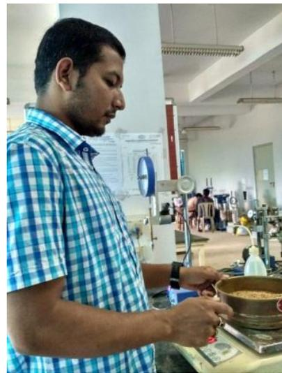
Figure : During the laboratory experiment for particle size distribution analysis of the soil samples collected from field
