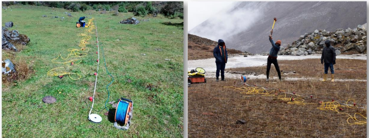
446 447 Figure 15: MASW survey at a location (MASW5) between Lachen and Thangu Valley (left) and 448 (MASW2) Changme glacial snout (right)
