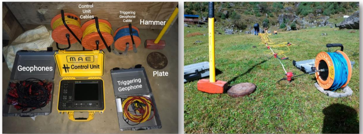
287 288 Figure 8: Photographs of MASW components (left) and field installation (right)
