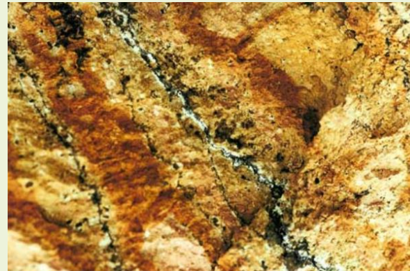
Clay vein formed along a deformed relict joint plane
