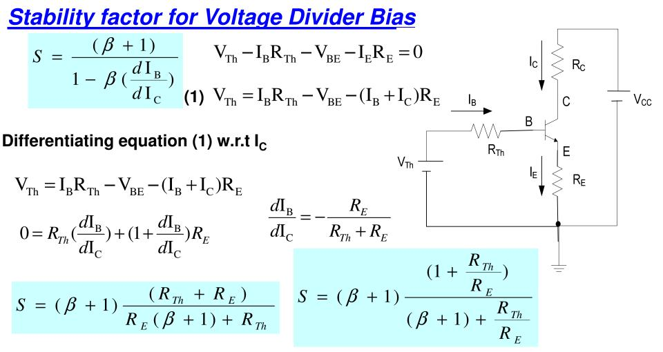
> For stability, S should be small which can be achieved by making  $R_{Th}/R_E$  small. For very small  $R_{Th}/R_E$ ; S = 1 (ideal case)
