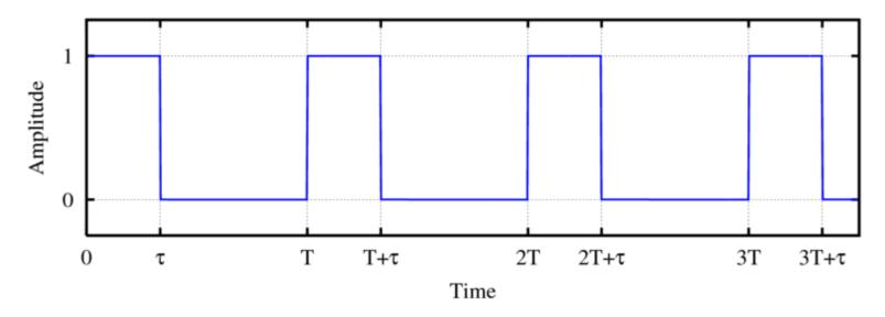
The pulse duration is  $\tau$ ; this is how long the pulse remains high (amplitude=1 in the figure). The pulse period is T ; this is the duration of one complete cycle, and is just the inverse of the frequency in Hz (f = 1/T).
