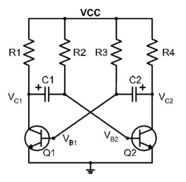
Consists of two amplifying devices cross-coupled by resistors and capacitors. Typically, R2 = R3, R1 = R4, C1 = C2 and R2 >> R1.
