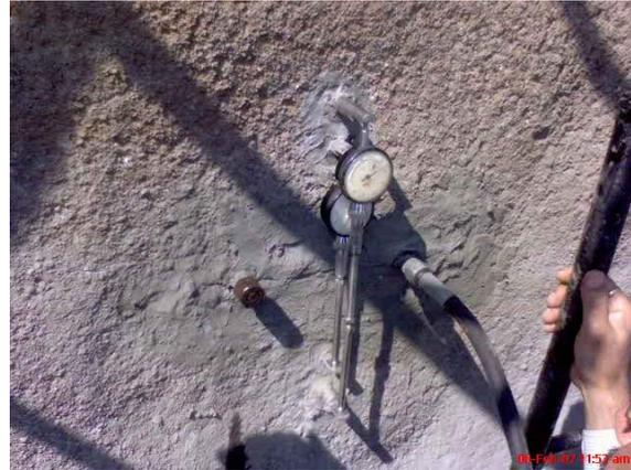
Fig. 2 Placing of dial gauge after fixing flat jack between the two pins
