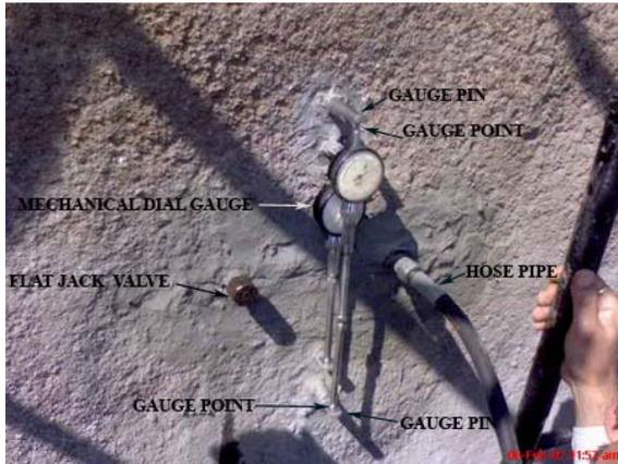
Fig. 3 View of embedded flat jack and four reference pins in the slot
