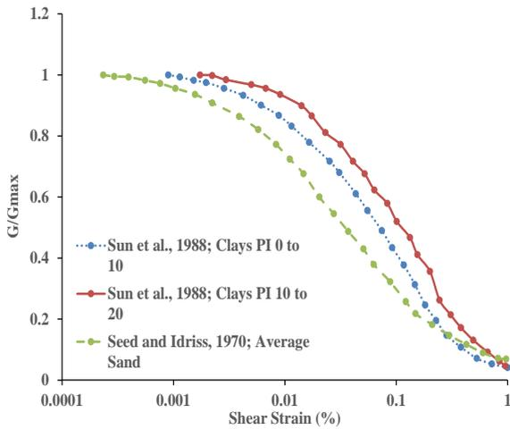
**Figure 3:**  $G/G_{max}$  curve for different soil types
