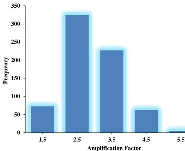
**Figure 6:** Plot of amplification factor versus frequency considering all the borehole analyses
