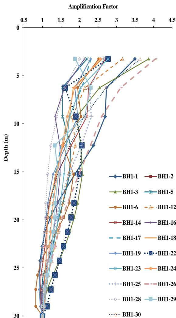
**Figure 5:** Revised amplification factor variation corresponding to Figure 1 after applying the three observations
