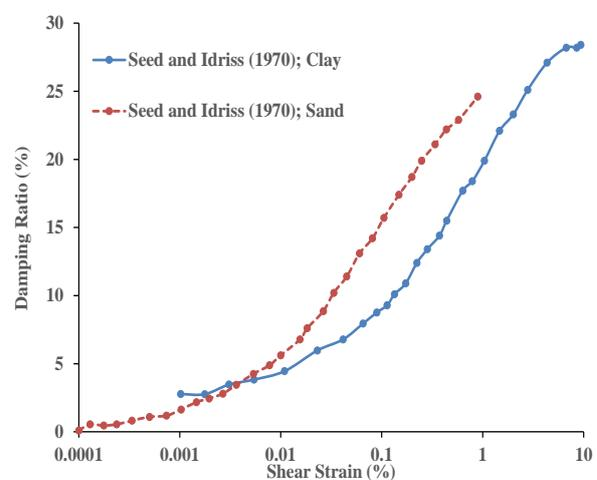
**Figure 2:** Damping ratio curves for different soil types
