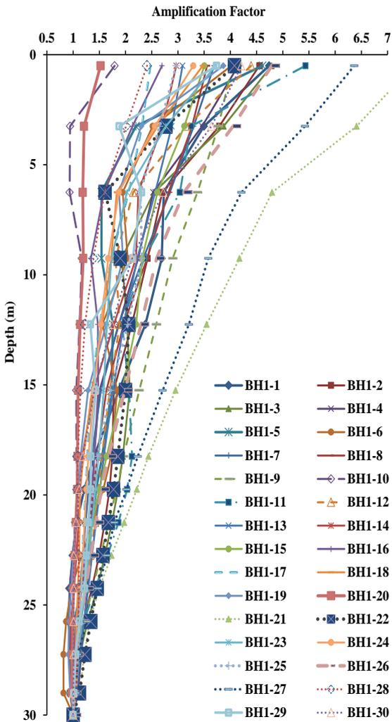
**Figure 4:** Typical plot showing the variation in amplification factor corresponding to selected ground motions
